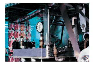
A patented quick start solution for reduced warm-up times and operating costs is sold separately as an option. Although the UV cassettes generate a high irradiance, the UV light as such is cold. Therefore, the packaging material is not heated. The disinfection method is thus perfectly suited to heat-sensitive materials such as plastic cups or heat sealing film. Due to their geometry, Premium UV modules are particularly well adapted to in-line filling machines with 4 to 12 rows of cups.
